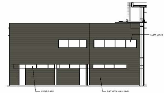
PARTIAL EAST ELEVATION
